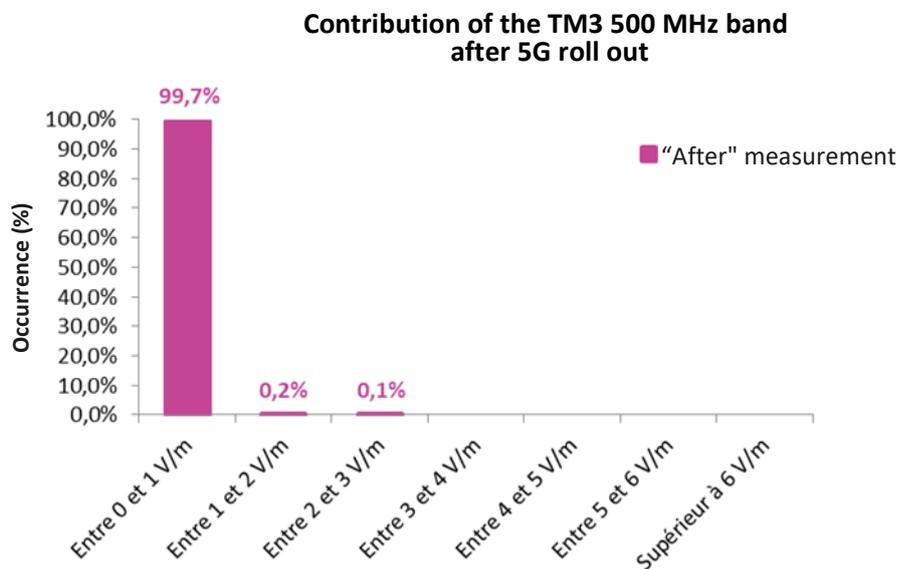
**Figure 15. Contribution of the 3 500 MHz band after 5G roll out estimated from 1 062 measurements**
