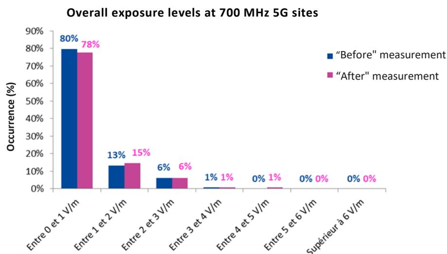
**Figure 9. Distribution of overall exposure levels before and after 5G roll out on 143 700 MHz sites**
