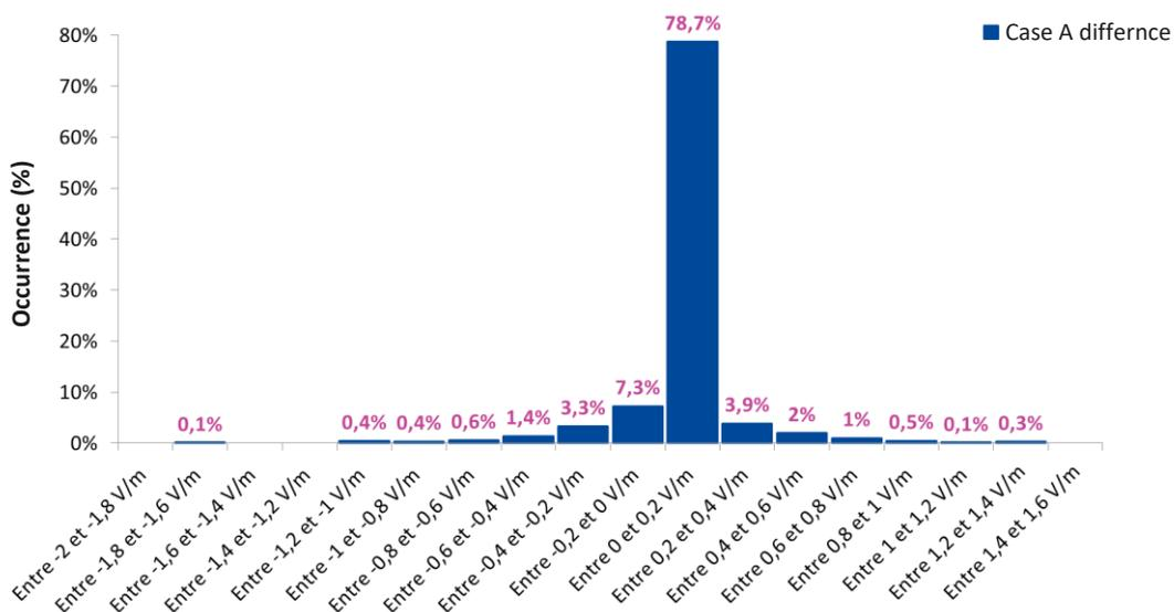
**Figure 18. Distribution of differences between overall exposure levels before and after 5G roll out on 1359 5G 3 500 MHz sites**
