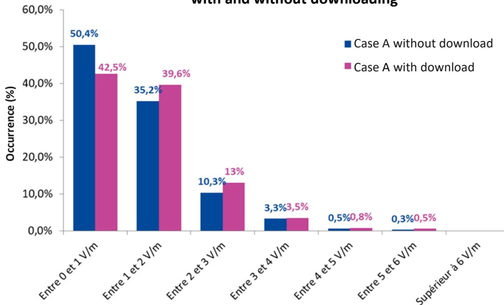
Figure 21. Distribution of the average level over 6 minutes from the specific measurement with 5G solicitation included in case A global exposure by calculation, and compared to the case A measurement "after" without specific network solicitation
