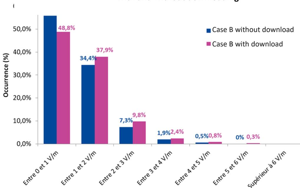
Figure 22. Distribution of the average level over 6 minutes from the specific measurement with 5G solicitation included in the case B overall exposure by calculation, and compared to the case B measurement "after" without specific network solicitation
