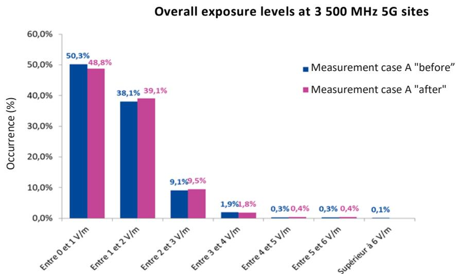
**Figure 17. Distribution of overall exposure levels before and after 5G roll out on 1359 3 500 MHz sites**
