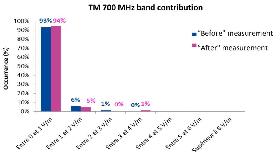
Figure 7. Distribution of exposure levels in the 700 MHz band before and after 5G roll out on 87 sites
