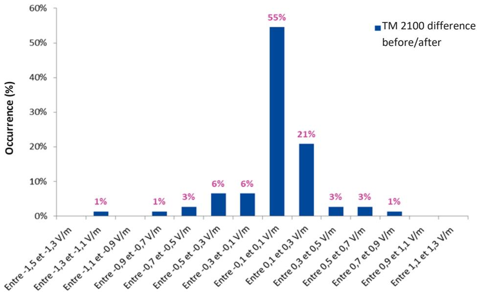
Figure 12. Distribution of differences between 2 100 MHz band contribution before and after 5G roll out at 772 100 MHz sites
