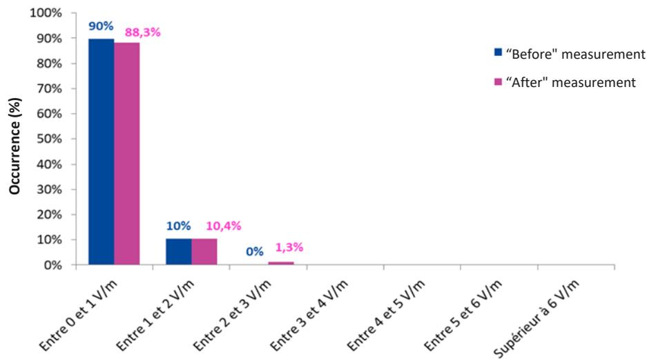
**Figure 11. Distribution of exposure levels in the 2100 MHz band before and after 5G roll out at 77 sites**
