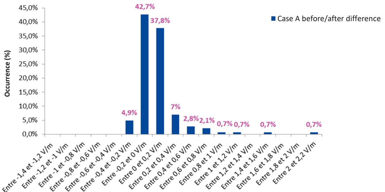
**Figure 10. Distribution of differences between overall exposure levels before and after 5G roll out on 143 700 MHz sites**
