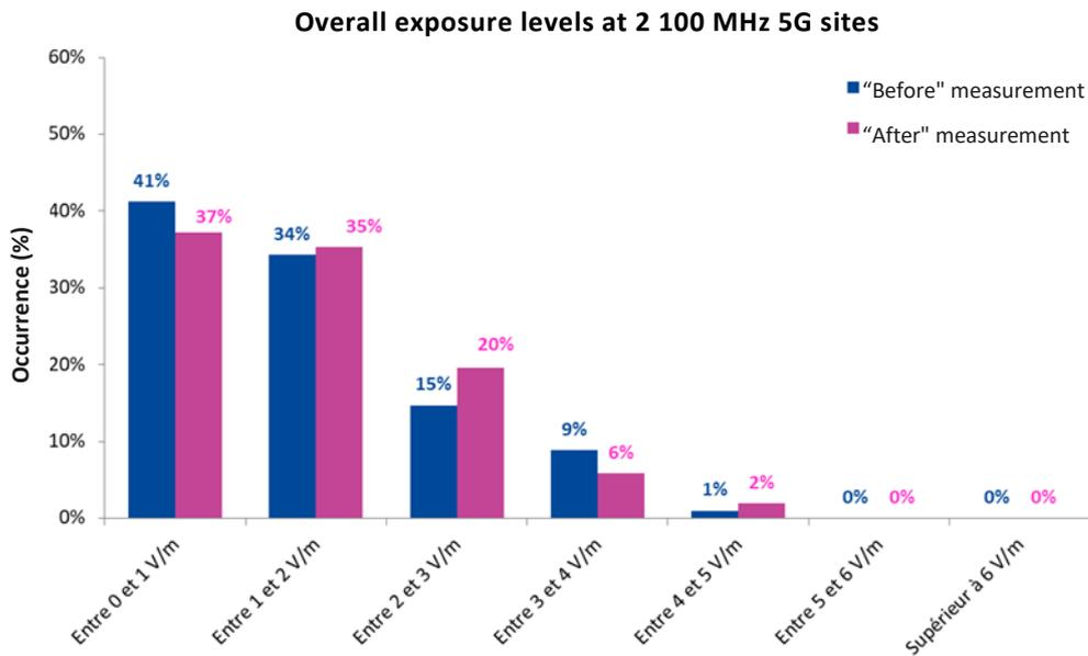
**Figure 13. Distribution of overall exposure levels before and after 5G roll out at 102 2 100 MHz sites**
