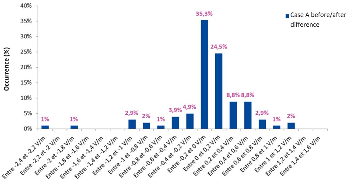
Figure 14. Distribution of differences between overall exposure levels before and after 5G roll out on 102 5G sites in the 2100 MHz band
