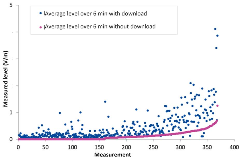
**Figure 20. Average field level over 6 minutes while downloading a 1 Gb file compared with the average level over 6 minutes without downloading**
