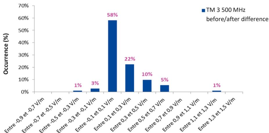
**Figure 16. Distribution of differences between 3 500 MHz band contribution before and after 5G roll out at 1113 500 MHz sites**
