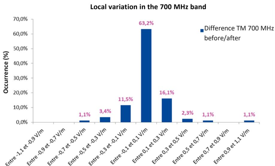
**Figure 8. Distribution of differences between 700 MHz band contribution before and after 5G roll out on 87 700 MHz 5G sites**
